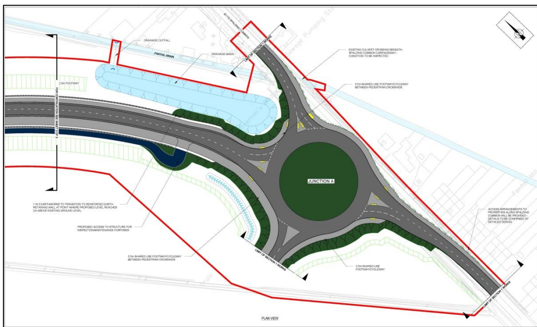
Section 1 – Proposed four-arm roundabout - proposed highway finishes
